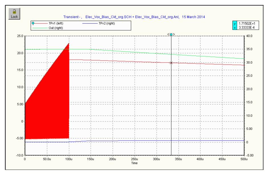
The next chart shows the same drive except a longer time scale of 25ms. Note that the output (green line) takes apx 8ms to fully turn-on, stays o for apx 4ms and then turns off heading for cutoff bias.
