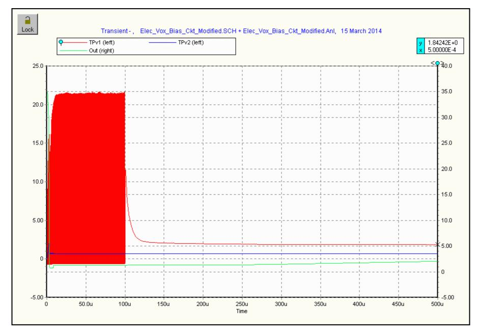
The drive signal (red) pulses is a 2Mhz @ 40 watts. Works with as low as 10W RF drive. With Q2's added-gain, the ckt can be driven with low power The output (green) attains operating bias in < 10us after RF drive signal is introduced. The tube stays biased for the dead time interval as the chart below shows.
