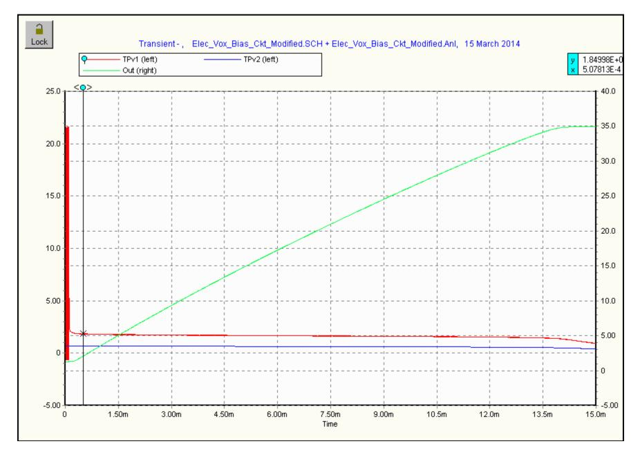
From Ous to 15ms (chart above), the EVB ckt starts to turn off at 500us time point. It takes apx 12ms to return to cutoff bias. This is perfect for CW users but works equally well for SSB where long hang-time is not desired.
