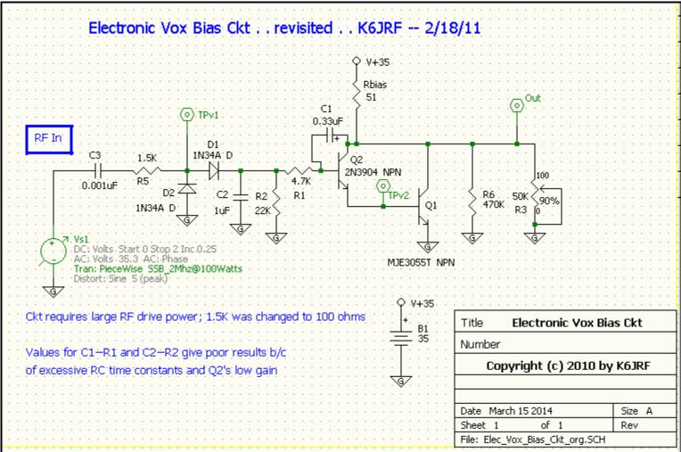
The time-constant of C1-R1 and C2-R2 are much too long for reliable ckt operation. These ckt values result in an extremely slow response time as the chart on the next page shows. The attenuating resistor, R5 had to be changed to 100 ohms to get the ckt to respond to 2Mhz signal @ 100 watt: drive!! That's due the poor choice of C1-R1 and C2-R2 RC time constants and the low gain of the main transistor "switch", Q2.
