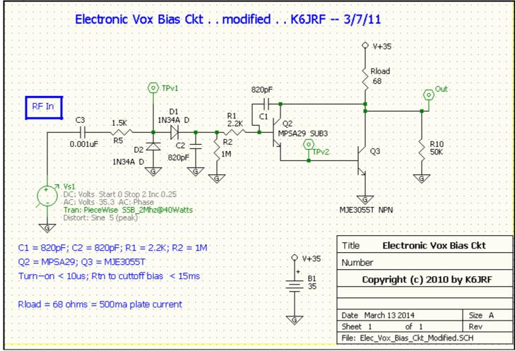
The 5Spice ckt values were modified or replaced with ckt values that make it work as a "real" Electronic Vox Bias ckt. New values for C1 and C2 = 820pF as well a replacement for Q1, MPSA29 have been employed. Resistor R2 stays the same. The ckt, with short time constant, can be used for either "CW" or "SSB" operation.
